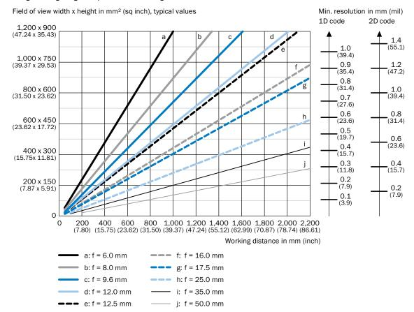
For S-mount and standard C-mount lenses, distance rings are needed for working distances shorter than approximately 10 times the focal length. For Compact C-mount lenses, distance rings are not needed, but the integratable lighting cannot be used for distances shorter than 300 mm
