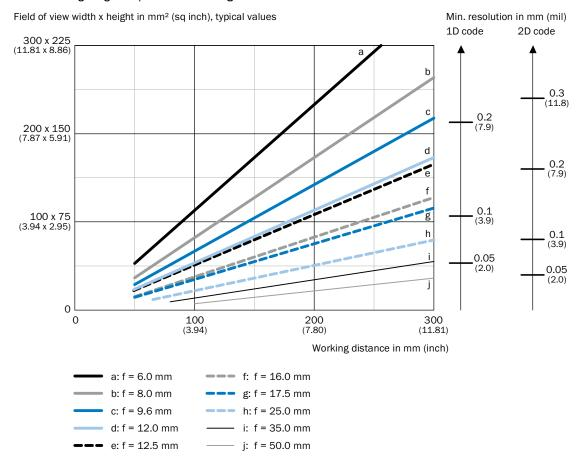
For S-mount and standard C-mount lenses, distance rings are needed for working distances shorter than approximately 10 times the focal length. For Compact C-mount lenses, distance rings are not needed, but the integratable lighting cannot be used for distances shorter than 300 mm
