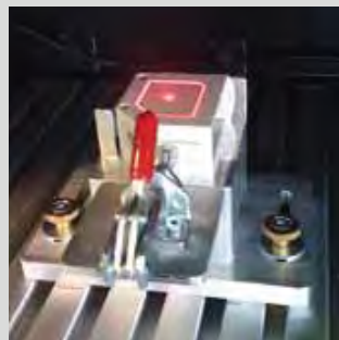
No identity crisis: All F 55 sensors are identified in the SensoPart production line using the latest laser marking devices. In contrast to standard inscription, laser marking is resistant to abrasion and cleaning, enabling an easy identification of sensors even after years of use.
